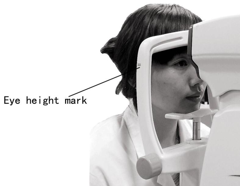
4. Use control bar to adjust the instrument to target the person's eyes. Through horizontal / vertical adjustment to locate eyes in the focus box.
